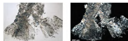
Figure 2: Fine samples under polarized light for conditions EXP 02 - LONGITUDINAL - 100X magnification - zero degree par - 75 degrees polarization
